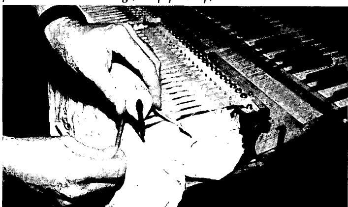
photo 15: hammer sanding (sandpaper strip)
