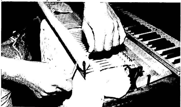
photo 14: hammer sanding (sandpaper strip)
